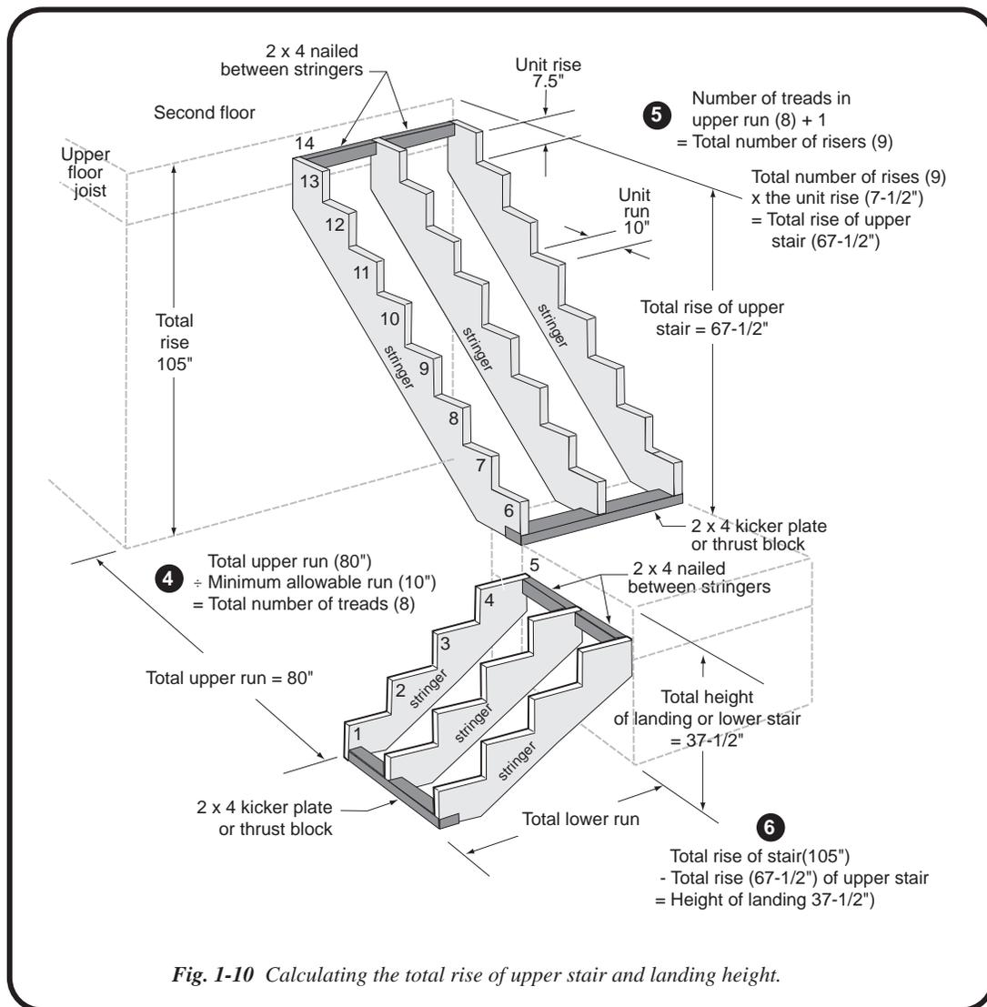
5. The L-shaped stair, like any other staircase, will start with a rise and end with a rise. Add one to the number of treads (8+1) determined for the upper stair and multiply this by the unit rise (7-1/2") to determine the total rise for the upper stair.
