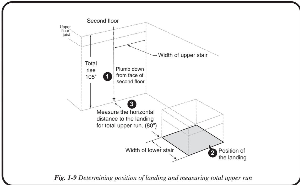
2. Determine position of landing and then draw the landing out on the first floor.
