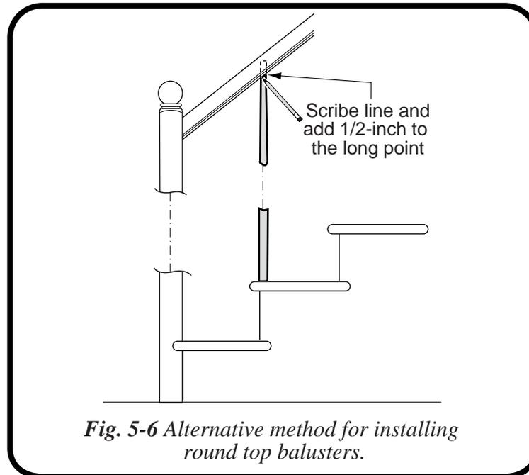
5. Add 1/2-inch to the longest point of this line and make a square cut on this mark with a miter saw.
