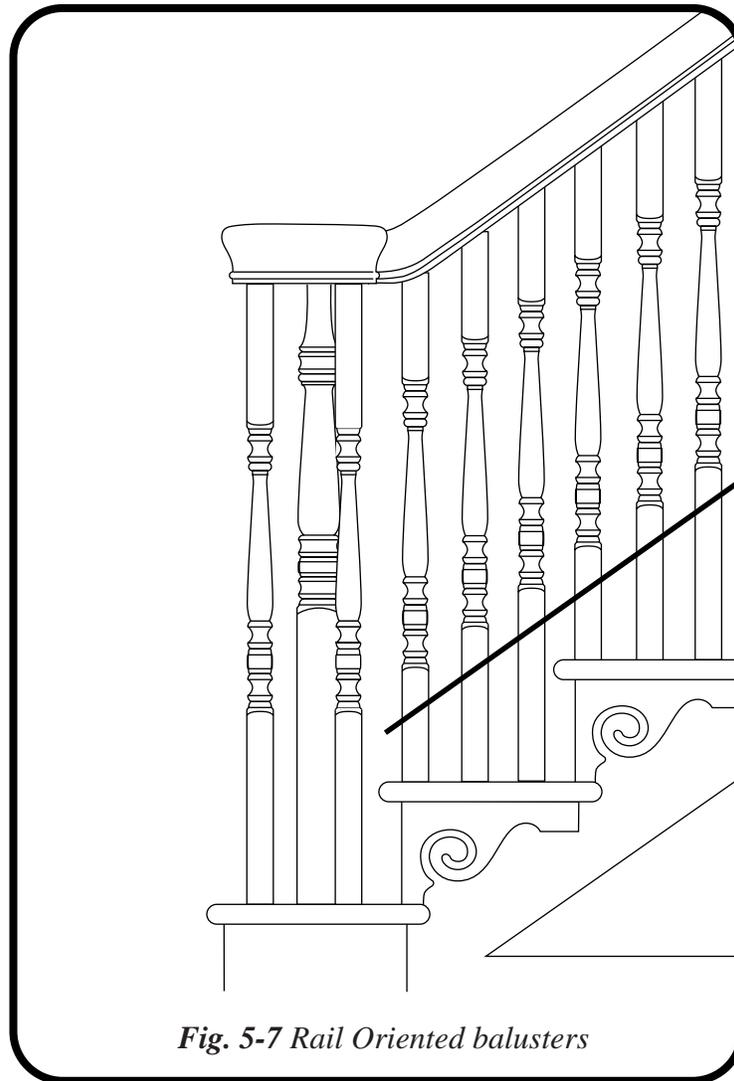
*Fig. 5-7 Rail Oriented balusters*
