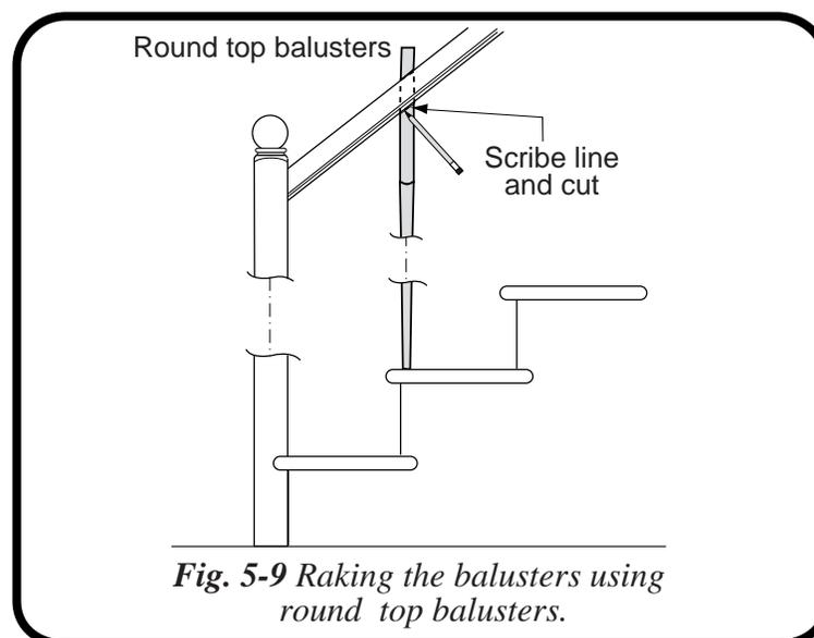
2. Center the bottom of the baluster with the hole in the bottom of the rail and scribe a line on the baluster along the pitch of the rail using the bottom of the rail as a guide. Please note Fig. 5-9 on the previous page.
