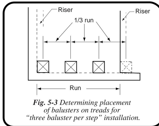
**Note: Most building codes dictate that baluster placement must not allow a 4-inch sphere to pass through it. Consult local building codes for exact requirements.**
