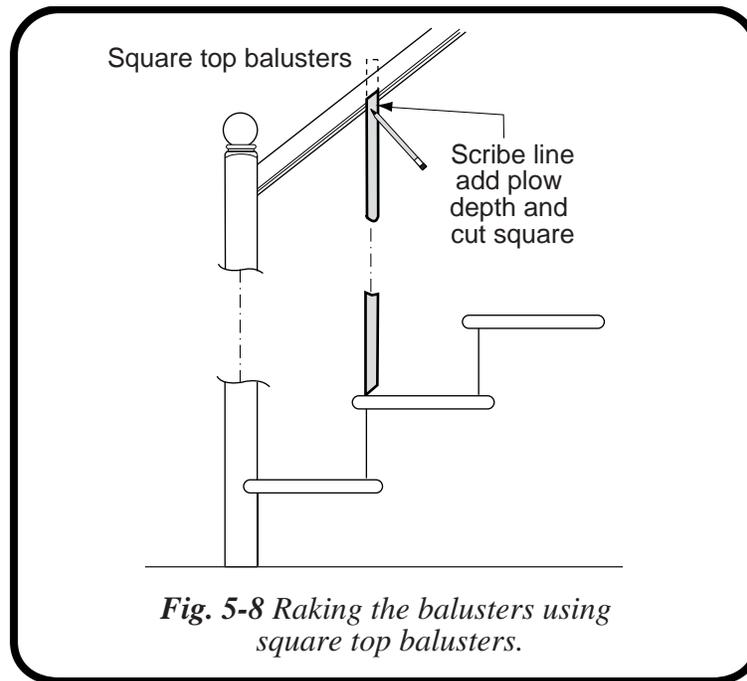
5. From this mark, cut the balusters square and add a dowel to the bottom as directed above.
