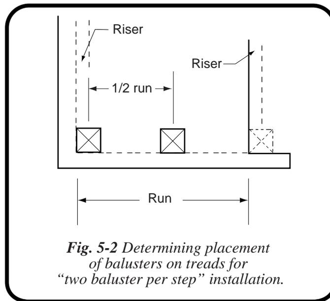
In the “three baluster per step installation” the placement is calculated the same way, except you must take the run and divide by three. Please note Fig. 5-3 here.
