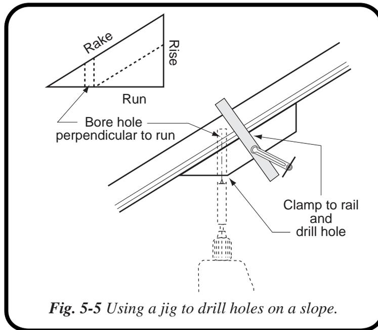
*Fig. 5-5 Using a jig to drill holes on a slope.*
